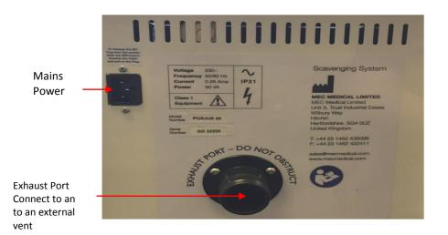
To release IEC plug from the socket. Slide the red button on the plug towards the cable and remove the plug from the unit.
